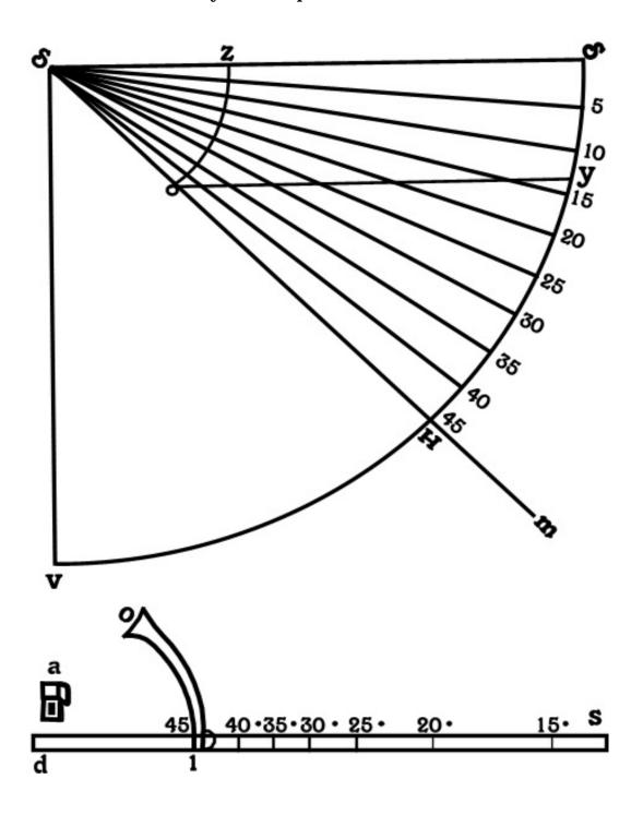
hole made for the staffe to runne in, as other staues haue, also there must bee a plate of brass with a soccat to be set to the cēter of the staffs, as is the figure *a*, in the midst wherof there must be a slitte, through which the sight must be conueied to the Horizon, and this plate must receive the shadowe of the transversary, and so the staffe is finished.
