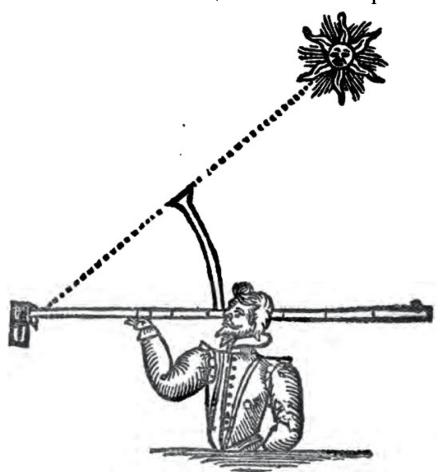
must be turned to that part of the Horizon which is from the Sunne, and with your backe toward the Sunne, by the lower edge of the halfe crosse, and through the slitte of the plate you must direct your sight onely to the Horizon, and then moouing the transuersary as occasion requireth, vntill the shadow of your vpper edge of the transuersary doe fall directly vpon the said slitte or long hole, and also at the same instant you see the Horizon through the slitte, and
